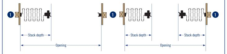
Stock Depth Ratio: 125mm per lineal metre of opening, PLUS 64mm for the lead post. NOTE. For Bi-Parting doors use half the opening width.
