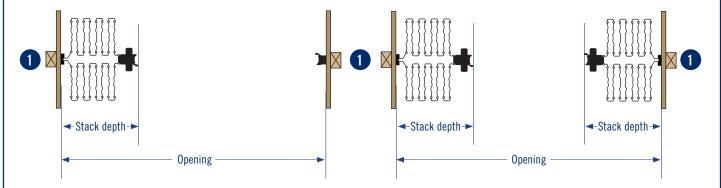
Stack Depth Ratio: 146mm per lineal metre of opening, PLUS 152mm for the lead post. NOTE. For Bi-Parting doors use half the opening width.
