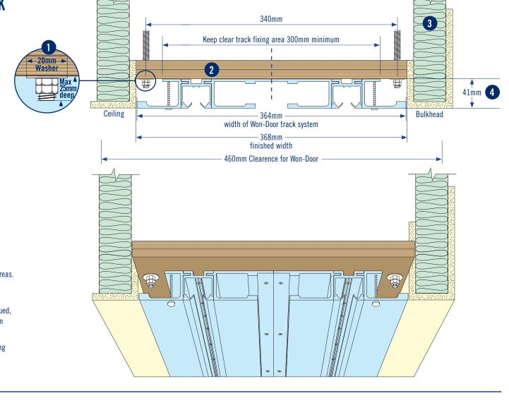
1. 10mm threaded rod with nuts and washers by main contractor.
