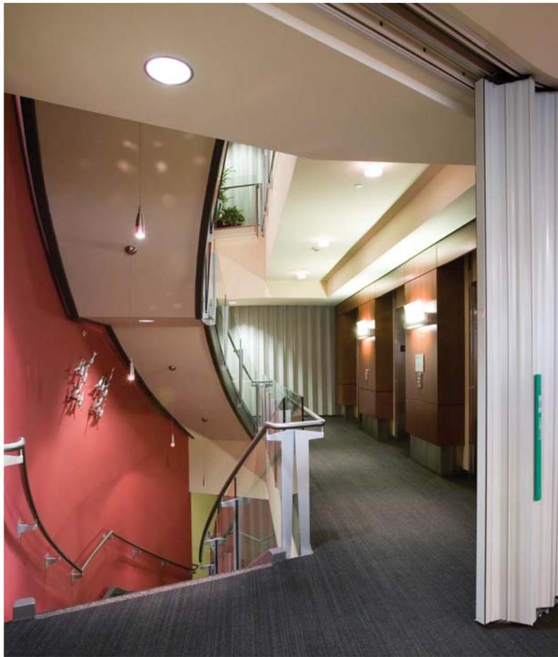
The same Won-Door FireGuard fire doors are used in this elevator lobby/ stairwell to satisfy two code-enclosure requirements – protection of a vertical opening as well as elevator lobby separation.
